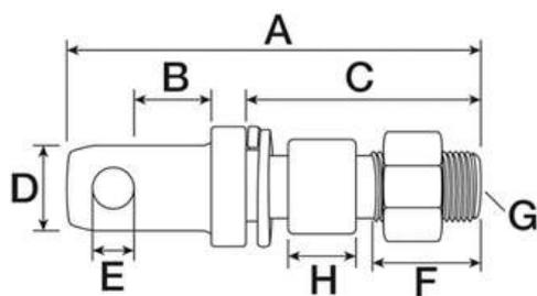
**Ø 22mm - A 104mm - C 60mm - Stabilisatorbolzen**
